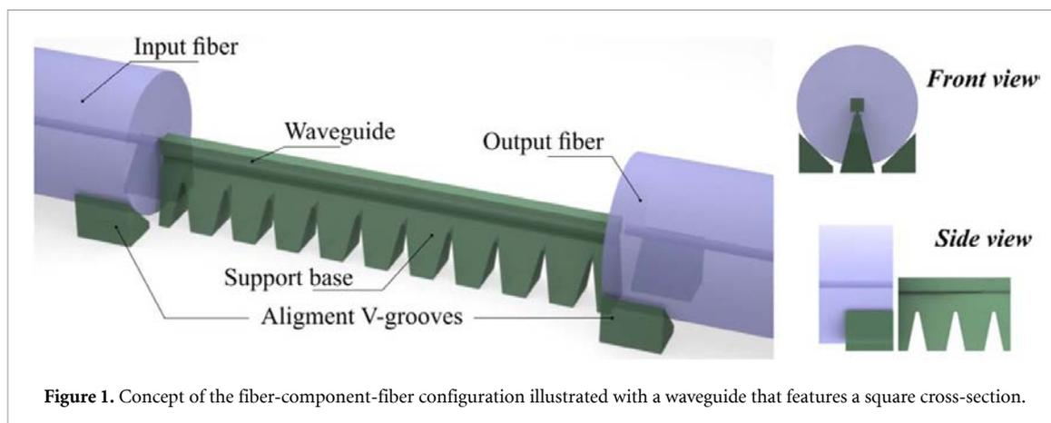
**Figure 1.** Concept of the fiber-component-fiber configuration illustrated with a waveguide that features a square cross-section.
