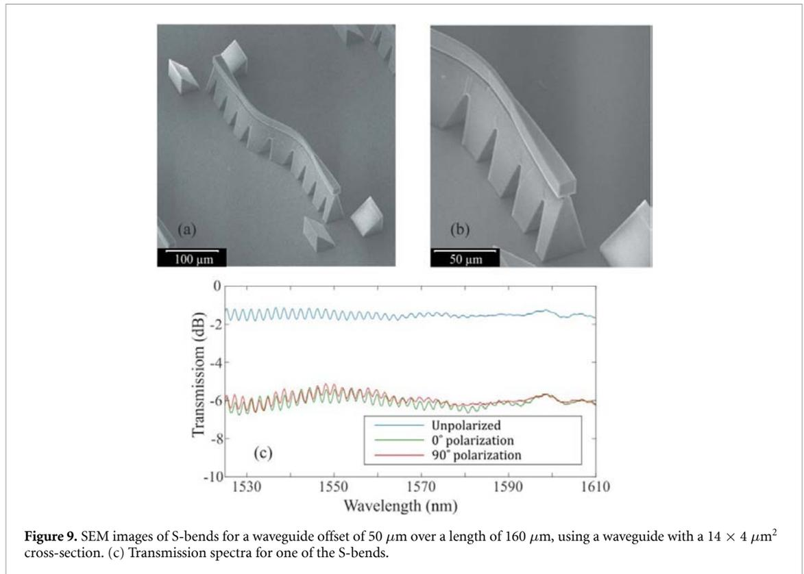
**Figure 9.** SEM images of S-bends for a waveguide offset of  $50\ \mu\text{m}$  over a length of  $160\ \mu\text{m}$ , using a waveguide with a  $14 \times 4\ \mu\text{m}^2$  cross-section. (c) Transmission spectra for one of the S-bends.
