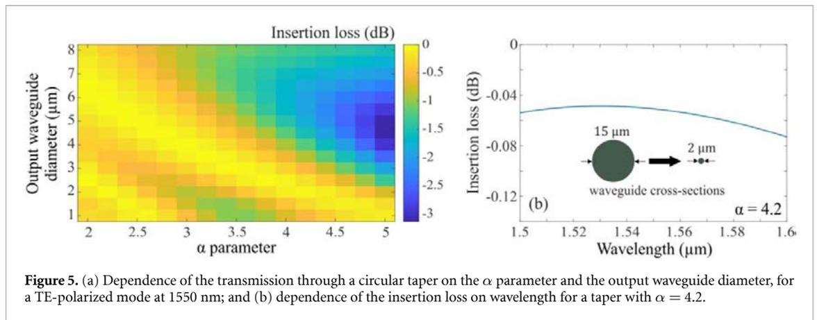
**Figure 5.** (a) Dependence of the transmission through a circular taper on the  $\alpha$  parameter and the output waveguide diameter, for a TE-polarized mode at 1550 nm; and (b) dependence of the insertion loss on wavelength for a taper with  $\alpha = 4.2$ .
