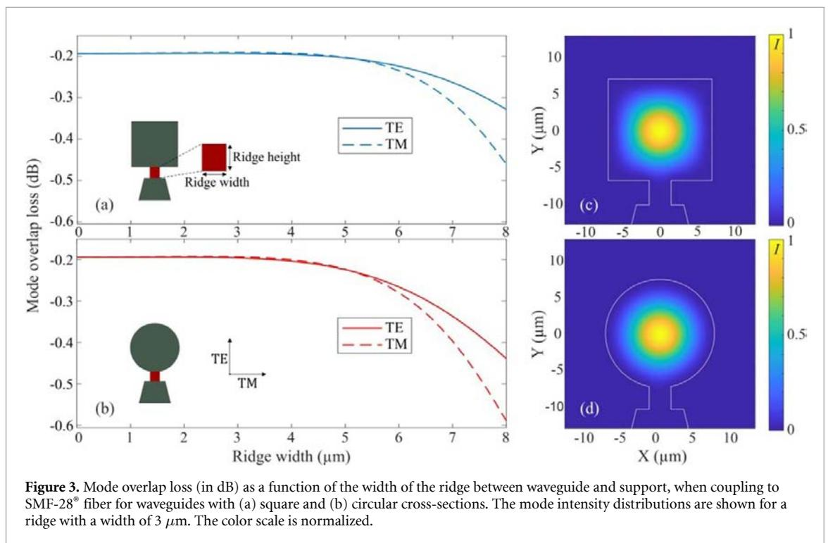
**Figure 3.** Mode overlap loss (in dB) as a function of the width of the ridge between waveguide and support, when coupling to SMF-28<sup>®</sup> fiber for waveguides with (a) square and (b) circular cross-sections. The mode intensity distributions are shown for a ridge with a width of 3  $\mu\text{m}$ . The color scale is normalized.
