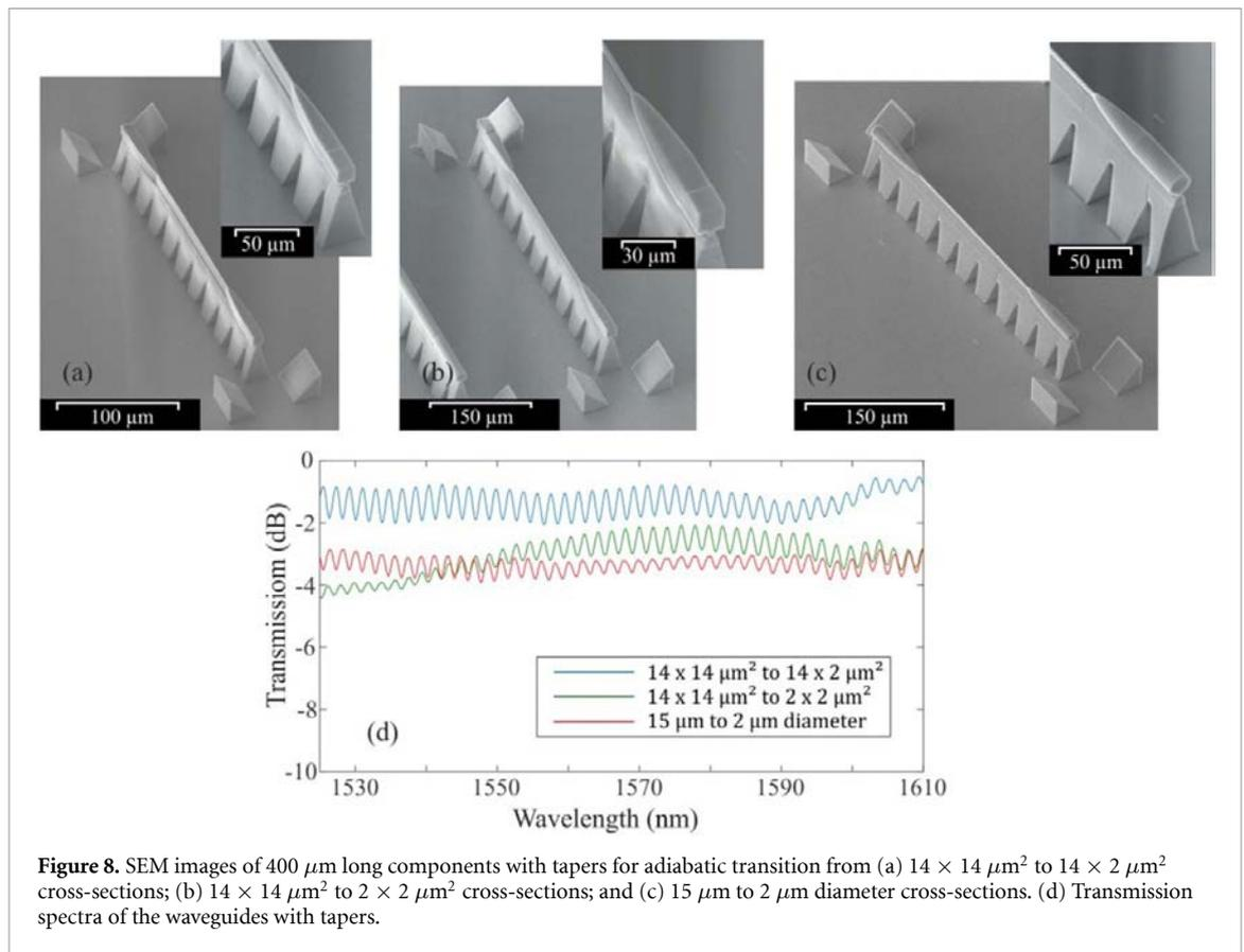
**Figure 8.** SEM images of 400  $\mu\text{m}$  long components with tapers for adiabatic transition from (a)  $14 \times 14 \mu\text{m}^2$  to  $14 \times 2 \mu\text{m}^2$  cross-sections; (b)  $14 \times 14 \mu\text{m}^2$  to  $2 \times 2 \mu\text{m}^2$  cross-sections; and (c)  $15 \mu\text{m}$  to  $2 \mu\text{m}$  diameter cross-sections. (d) Transmission spectra of the waveguides with tapers.
