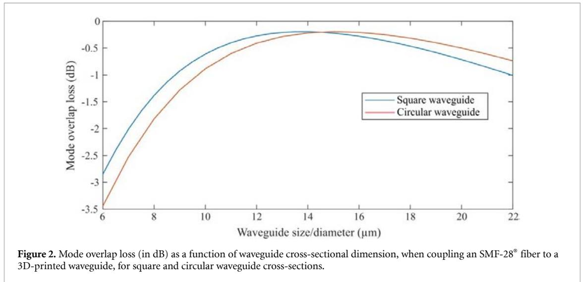
**Figure 2.** Mode overlap loss (in dB) as a function of waveguide cross-sectional dimension, when coupling an SMF-28<sup>®</sup> fiber to a 3D-printed waveguide, for square and circular waveguide cross-sections.
