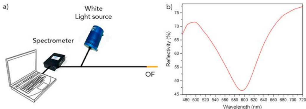
**Fig. 3.** (a) Scheme of the optical fiber probe connected to a spectrometer and a white light source (480–720 nm). The device is portable and can be connected to a laptop. (b) Gaussian SPR curve obtained with the gold-coated OF in PBS. (For interpretation of the references to colour in this figure legend, the reader is referred to the Web version of this article.)
