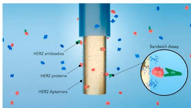
**Fig. 2.** Artistic view of the gold coated unclad fiber used to specifically detect HER2 molecules (in red) through SPR, with antibodies amplification in a sandwich configuration (in green). Thiolated aptamers are immobilized on the gold surface to target HER2. (For interpretation of the references to colour in this figure legend, the reader is referred to the Web version of this article.)
