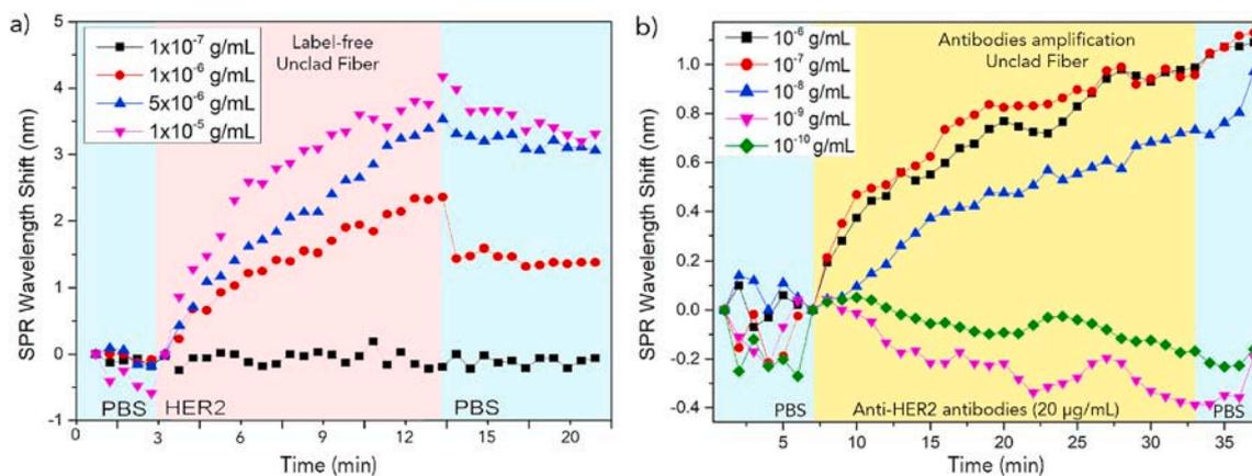
Fig. 6. (a) Evolution of the SPR-dip minimum in PBS, HER2 proteins, and PBS after the immersion in HER2 solution. (b) Evolution of the SPR-dip minimum in PBS, in antibodies (anti-HER2), and in PBS after amplification. Each curve represents one probe per test.
