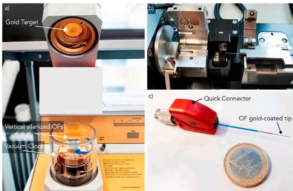
**Fig. 1.** (a) Picture of the gold sputter-coater. Optical fibers were placed vertically inside the vacuum chamber. The quartz microbalance is at the level of the lower stage in the vacuum clock. (b) Picture of the optical fiber cleaving machine, to cut the 400  $\mu\text{m}$ -diameter optical fibers. (c) Picture of the OF-SPR probes inside a quick connector. (For interpretation of the references to colour in this figure legend, the reader is referred to the Web version of this article.)
