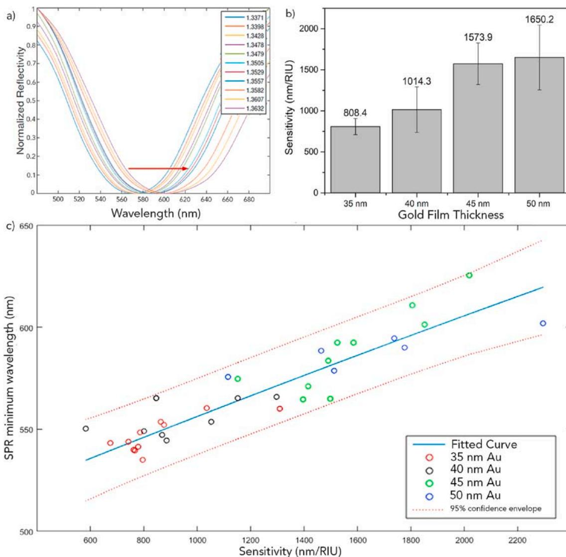
**Fig. 4.** (a) Evolution of the normalized spectrum in growing LiCl concentrations (RI change). (b) Evolution of the sensitivity as function of the gold film thickness (mean  $\pm$  sd). (c) Evolution of the SPR lambda 0 wavelength in PBS with different probes coated with growing gold film thicknesses (Fitted curve and 95% confidence envelope). (For interpretation of the references to colour in this figure legend, the reader is referred to the Web version of this article.)
