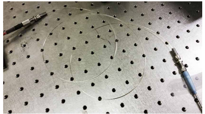
Fig. 7. A section of bioPOF with SMA905 connectors leading to optical fibers.
